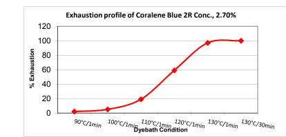
(Dyeing at different dyebath temperature on polyester fabric at pH 4 adjusted with Levocol 4398)
