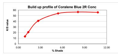
(Exhaust dyeing different depth at 130<sup>°</sup>C temperature for 45 min on polyester fabric at pH 4 adjusted with Levocol 4398)
