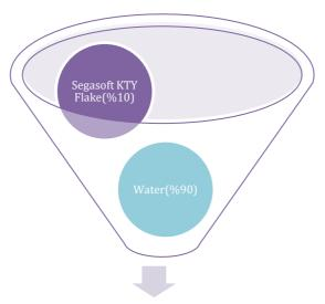
Add Segasoft KTY Flake at the specified rate to hot water brought to 80°C in advance. Addition should be done gradually temperature should not fall below 80°C. Then stir it continuously while cooling to room temperature in order to obtain a homogenous appearance.
